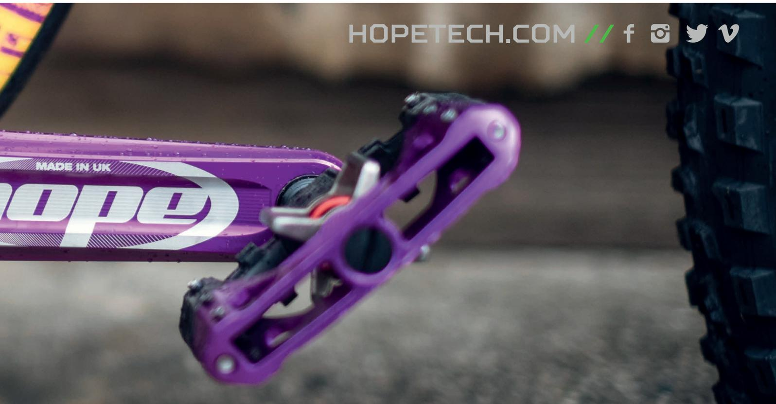
Added to this we CNC machine the arms from forgings which gives them immense stiffness and strength. The arms also have a splined mounting for spiders and direct mount sprockets giving excellent versatility. The spiders are available in either single (104 BCD) or double (64/104 BCD) ring configuration
