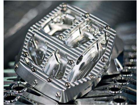
A right hand pedal body after first side machining.
