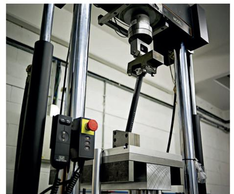
The HOPE Instron dynamic loading test bed testing an Eternity seat post.
