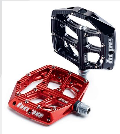
The pedals feature a fully CNC machined platform out of 2014 T6 Aluminium alloy with anodised finish (All 6 Hope colours). The axle is made of high strength Cr-Mo, heat treated and plated. The platform is slightly concave in shape and is supported by one Norglide bush and 3 cartridge bearings in a fully sealed chamber to ensure a long lasting and maintenance free running. The 20 replaceable pins per pedal will provide excellent traction and grip.
