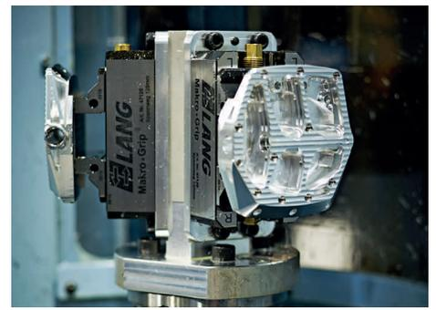
Each body is machined using simultaneous 5 axis machining.
