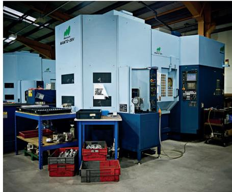
The 5 Axis Mam CNC takes 28 minutes to machine each pedal body.
